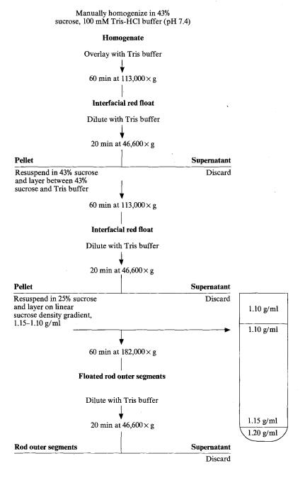
Outline of the procedure for obtaining rod outer segments from a homogenate of 100-120 bovine retinas.
